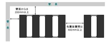
•Each abserver® moves a maximum of around 200mm horizontally in all directions during an earthquake. Secure a space more than 200mm from the obstacles such as a wall or the pillar and the side of abserver® or its load (depending on which is extrudes the most horizontally). •While abserver® is designed to oscillate at the same frequency and direction, regardless of load weight, during an earthquake, we nonetheless recommend an allowance of 400mm between adjacent abservers®.
